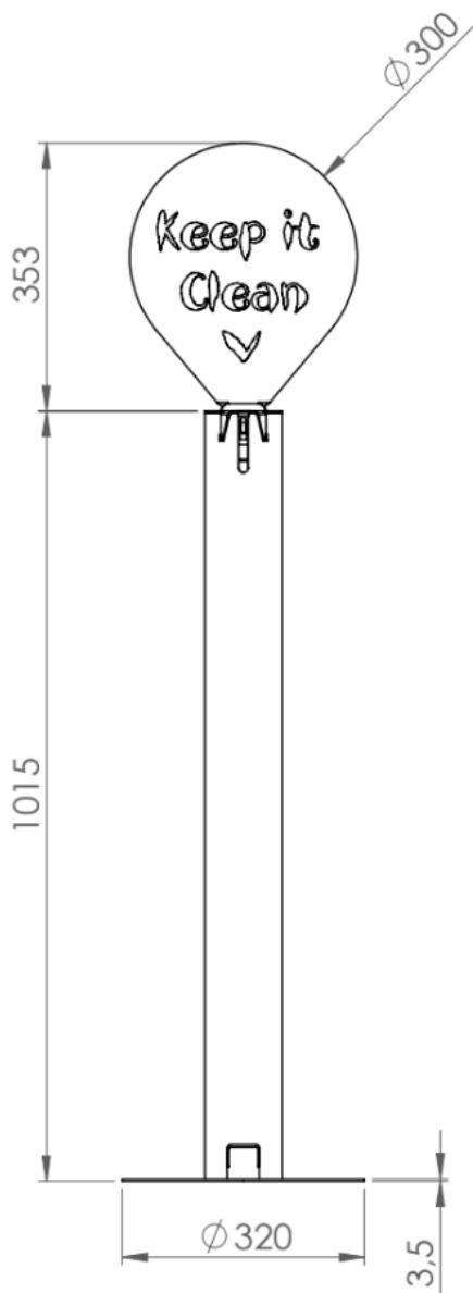
A robust hand sanitiser unit with concealed 1L bottle and hidden mechanism.
